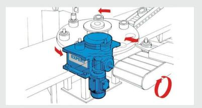
EXPERT globoidal rotary tables are equipped with hardened and ground globoidal cams and cam actuators.
